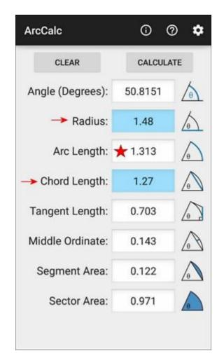
The L+G chord length value (1.27) and the measured radius (2.96/2) can be used in the above equations to obtain the estimated total number of land and groove sets (N) that could be fit abound the circumference of the sabot using the calculated L+G arc length (1.313):
