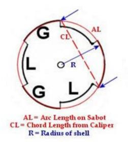
Sabot of typical 3 lands and groves rifling on the end of a rifled projectile. Using ArcCalc, the Arc Length (AL) of a single pair of rifling lands and grooves found on the projectile's sabot can be found from its measured Chord length (CL) and the radius of the projectile. Using these results the total number of lands and groove rifling sets can be estimated. This can then be used to identify the firing rifle.
